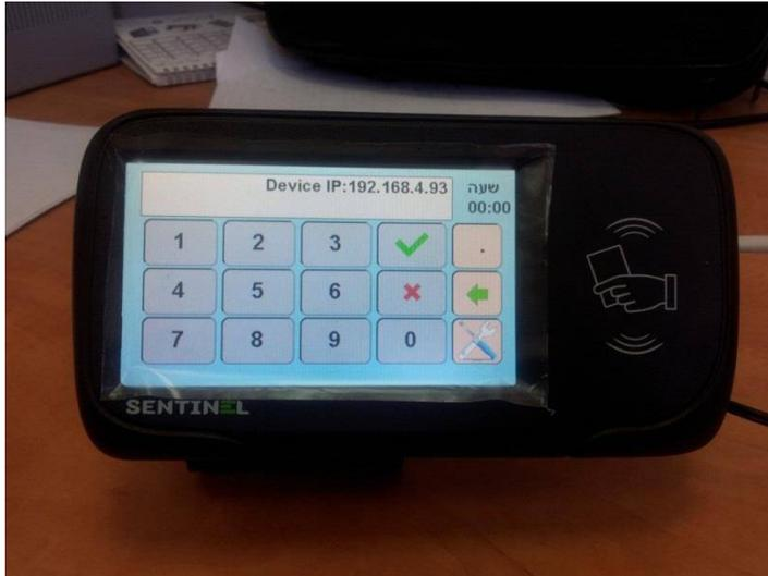
4. If you prefer dynamic IP address for the controller, then press settings icon to navigate the settings menu till you reach "DHCP Enable" item, then simply type the "1" and press "OK".
